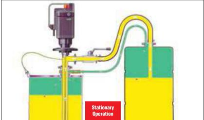
Concern about air pollution has never been so widespread as it is today. Acting on its sense of environmental responsibility, Lutz has further developed its emission proof drum adapter as a complete gas displacement system. Harmful gases and vapours created when transporting hazardous media remain practically in a closed system while themselves ensuring the necessary pressure compensation.
